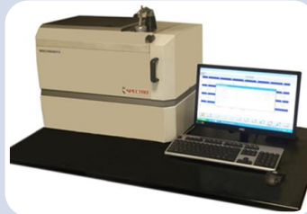
Spectrometer (determination of the chemical composition)
