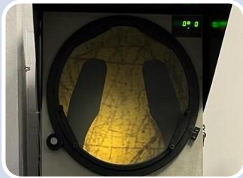
Optical profile projector (Dimension measure & validation)
