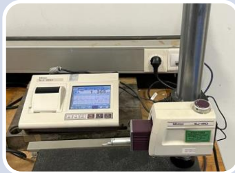
Roughness- meter (Roughness measure & validation)
