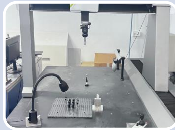
3DCMM machine (Dimension measure & validation)
