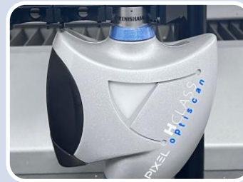
Optical scanner (Dimension measure & validation)
