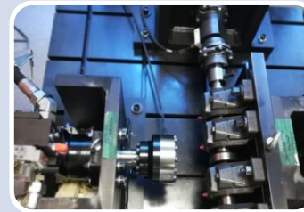
Biaxial Moog testing bench (Fatigue tests able to reproduce RLD)
