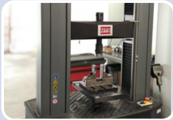
MTS insight static machine (Static measurements)
